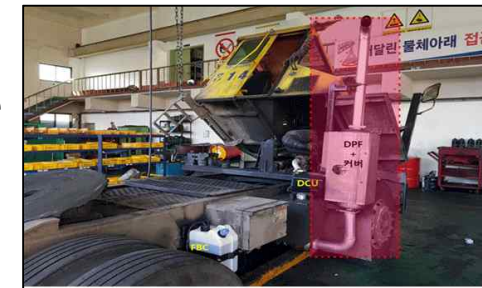
< YT DPF installation >
