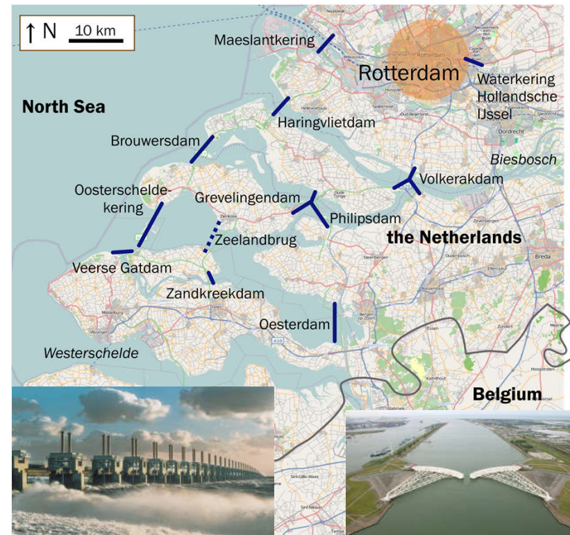
Delta Works: closed off major rivers with permant and flexible barriers to protect against flooding
